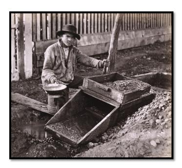
Moving the rocker back and forth, like a baby cradle, was similar to the motion of shaking a gold pan. The heavier gold would sink and the loose dirt and gravel would wash away.
